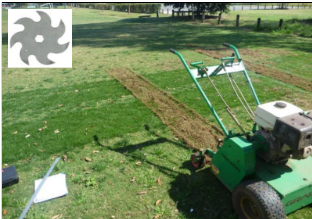
Plate 8. Graden® GS04 verticutter used to impose mechanical treatments at QSAC and Redlands United. Insert showing the style of tungsten carbide tip blade used with the Graden® verticutter..
